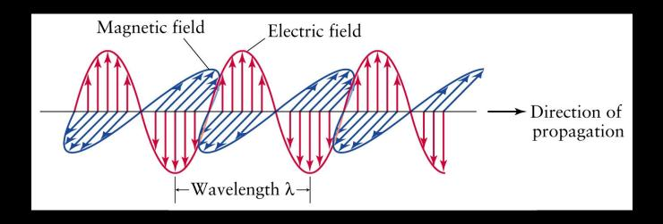
The changing magnetic field causes the electric field to change. When one field vibrates—so does the other.
